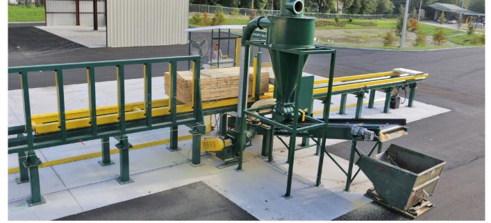
**Key Features and Options:** The Pacific Trail Accu-Cut has kerf collapse relief that protects the saw bar and chain, and the hitensile alloy saw bar provides long life. Options include fully automatic and remote controls, infeed staging for pre-loading, waste conveyors, and sawdust removal system.
